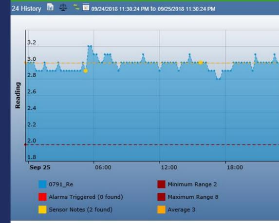
Figure 3: 24-Hour History Chart Showing Electronic Temperature Storage Log (all data points shown on the chart can be found in a table below the chart in the temperature monitoring software).
